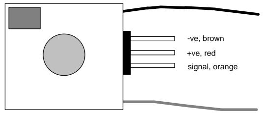
As soon as the LiPo Voltage Guard receives a valid throttle signal, the LED will go on, indicating that the device is ready to learn **the number of LiPo cells** that you are using. Move the throttle stick slowly up or down to a position where the LED flashing pattern matches the number of cells in the pack. Eg for a three cell LiPo pack, you want three flashes followed by a pause. For a ten cell LiPo pack, you want 10 flashes, followed by a short pause, etc.
